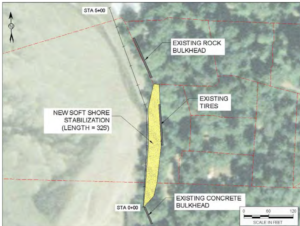
Figure 21. Alternative 1A project limits for soft shore protection concept of length 325 ft
