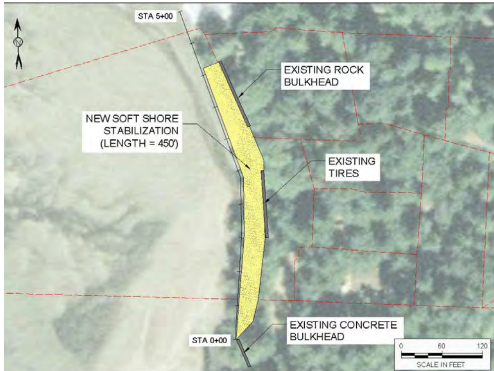
Figure 22. Alternative 1B project limits for soft shore protection concept of length 450 ft
